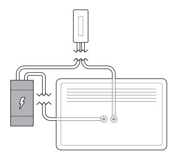
(Optional) Remove the transformer from its housing unit.
