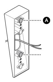
On stucco, brick, or concrete, use a 6 mm (1/4 in) masonry bit to drill holes for the included wall anchors.
