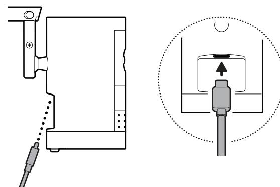
(Optional) If installing with a Quick Release Battery Pack, twist the battery cover to remove. Insert the battery and close.
